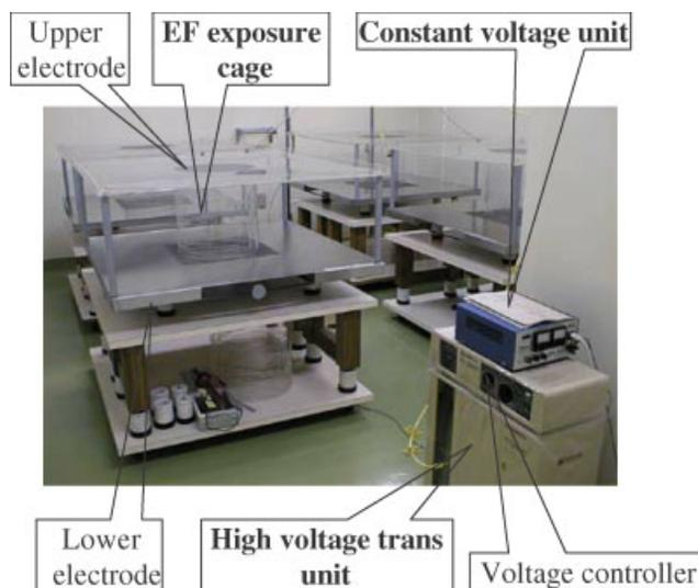
Fig. 1. The EF exposure system.
