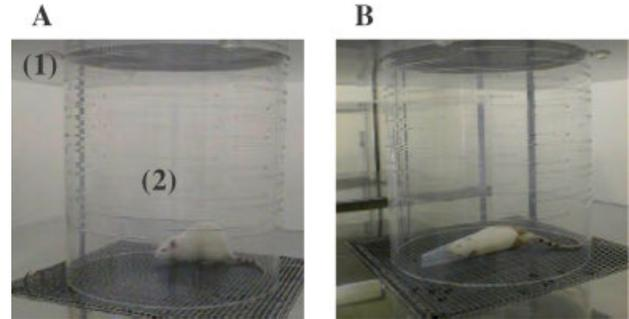
Fig. 2. The EF exposure cage. **A:** A cylindrical plastic cage (2) is placed between an upper (1) and a lower (3) stainless electrodes. The cylindrical cage has slits (length: 100 mm; width: 5 mm) around at intervals of 5 mm from each other. The slits prevent smudges, due to feces and saliva, disturbing formation of stable EF. **B:** A rat restricted by wrapping with a thin polyethylene sheet.
